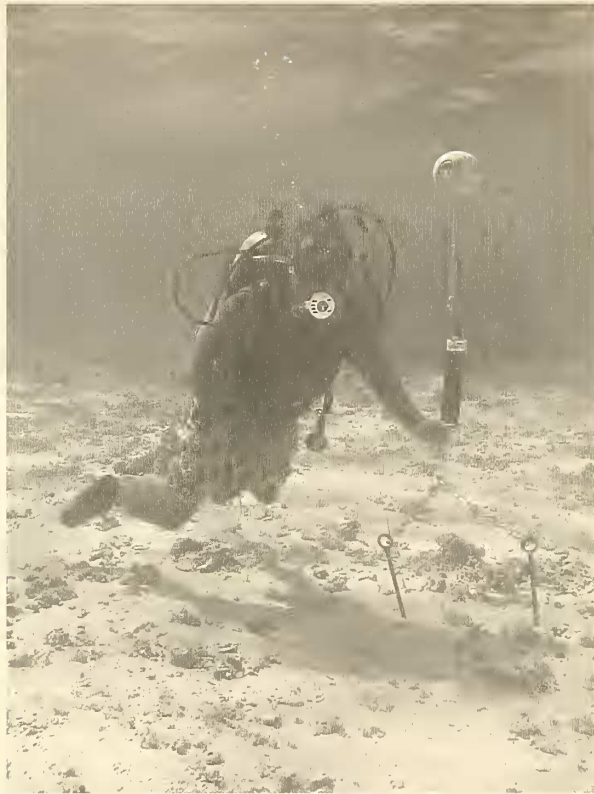
Figure 4. Diver with a VRI autonomous acoustic receiver anchored to the seafloor with sand screws.
